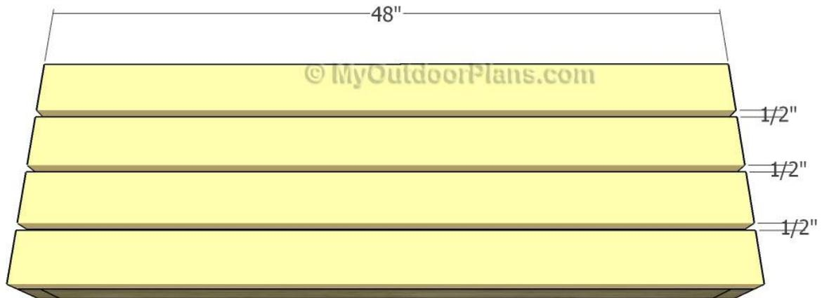
Next, you need to attach the 2×4 slats to the frame. Align the edges with attention and make sure the slats are equally-spaced. Drill pilot holes and insert 2 1/2" screws to secure the slats into place. You can place a 1/2" wood blog between the slats to get a professional result and equal gaps.
