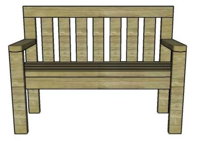
One of the last steps of the woodworking project is to take care of the finishing touches. Therefore, fill the pilot holes with wood putty and smooth the surface with 120-220 grit sandpaper. You can use wood plugs to fill the pocket holes as, well.
